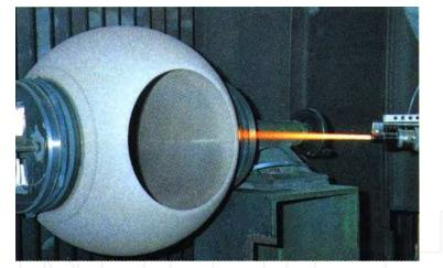
Fig. 11. HVOF coated spherical vane for nuclear industry Ducos (2006).
