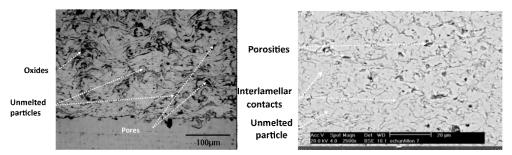
Fig. 4. (a) Stainless steel coating (304L) deposited by air plasma spraying on a low carbon (1040) steel substrate, (b) Y-PSZ (8wt%) coating deposited by air plasma spraying on a super alloy
