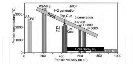
Fig. 2. Particle temperatures and velocities obtained in different thermal spray processes, as measured for high-density materials. The bar indicates the observed trend of recent developments (AS: Powder flame spraying, FS: Wire flame spraying, PS: Air plasma spraying, VPS: Vacuum plasma spraying, C.S.: Cold Spray) Gärtner et al (2006).
