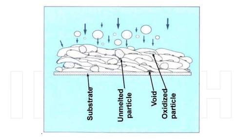
Fig. 3. Schematic cross section of a thermally-sprayed coating
