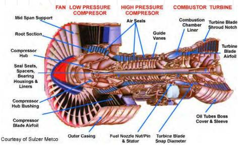
Fig. 10. Plasma-sprayed coatings on aircraft turbine engine parts (Courtesy of Sultzer-Metco)
