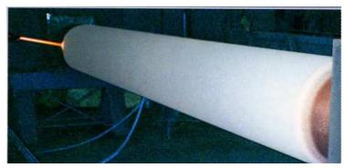
Fig. 8. Paper machine roll coated by NiCrBSi (self fluxing alloy) Vuoristo and Nylen, (2007).
