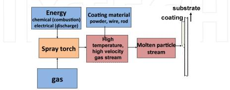
Fig. 1. Schematic of the thermal spray concept, Fauchais et al (2012)
