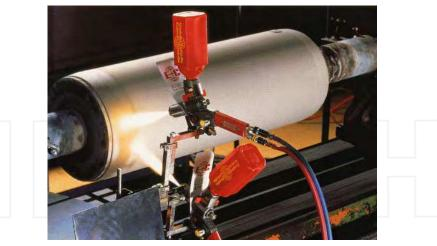
Fig. 7. Flame-coating of a cylinder used in food industry: 3-mm thick polyamide coating *Ducos* (2006).
