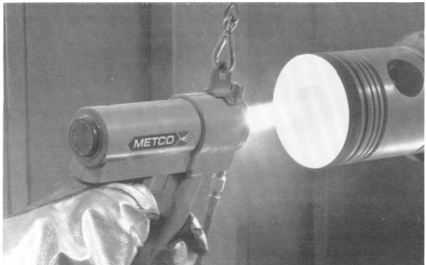
11.10 Plasma spraying a piston crown with a thermal barrier coating (courtesy Metco Ltd).
