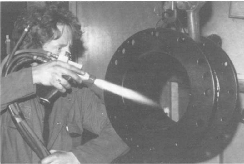
7.2 Naval exhaust muffler being thermally sprayed with nylon (courtesy Croboride Ltd).
