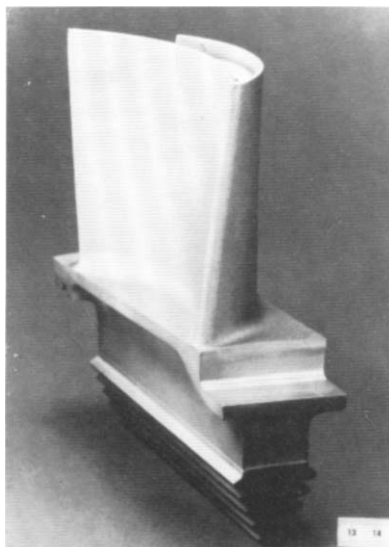
11.1 High temperature corrosion protection on turbine blade (courtesy Sulzer Metco Ltd).
