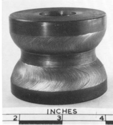
3.45 A TIG coating of a Co–Cr–W medium alloy on a guide roll, showing the smooth controlled profile of a mechanised weld deposit.
