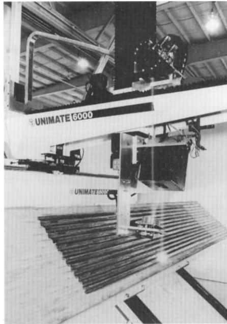
3.10 Laser cladding of waterwall panels (courtesy Praxair Surface Technologies Ltd).
