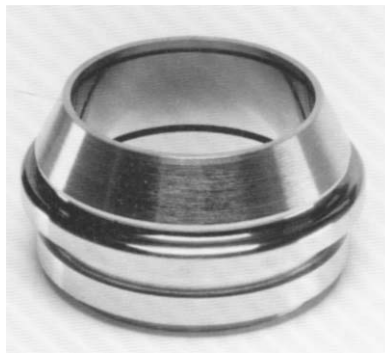
11.11 Can seaming roll of Co–Cr–W low alloy before coating with TiN by PVD (courtesy Deloro Stellite Group).
