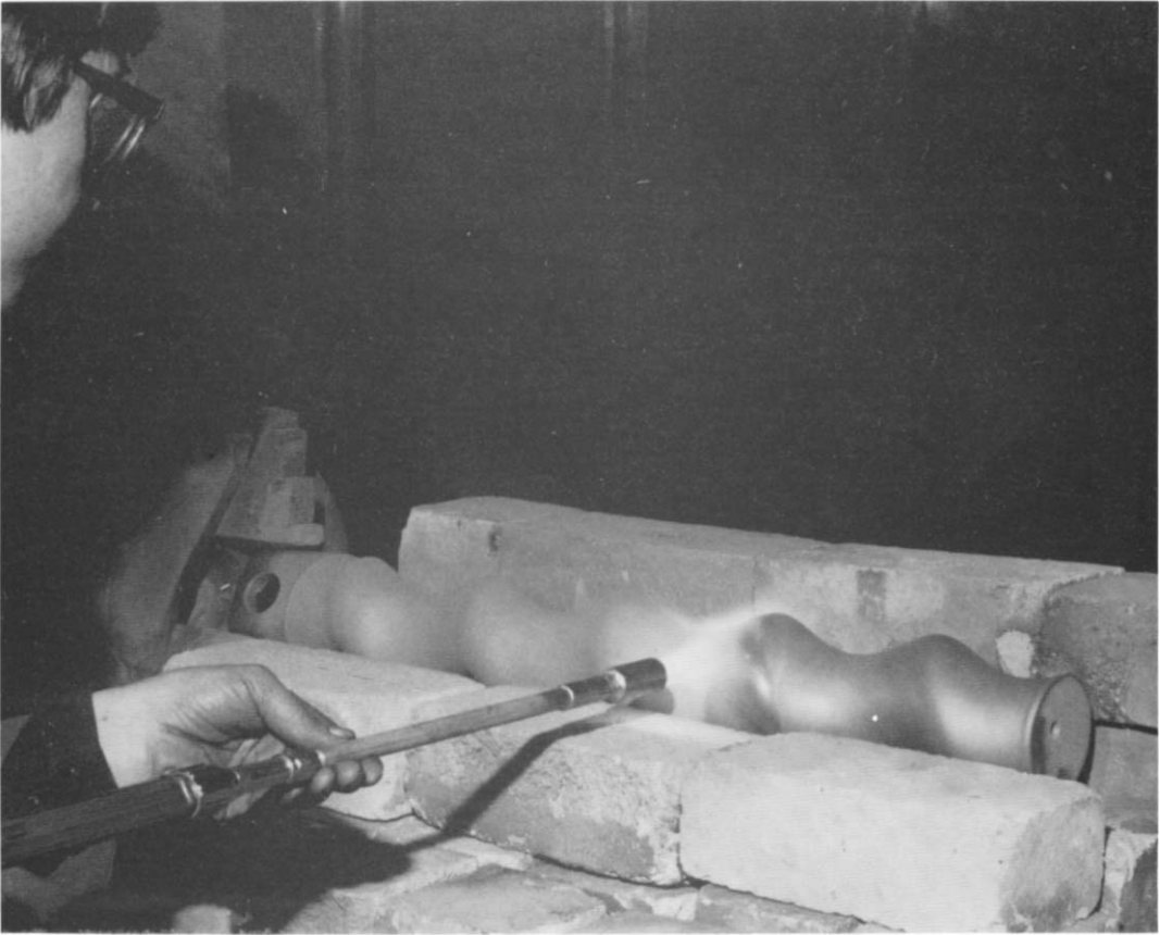
4.30 Manually fusing the thermally sprayed deposit of a Cr–Si–B alloy on the surface of a pump rotor (courtesy Deloro Stellite Group).
