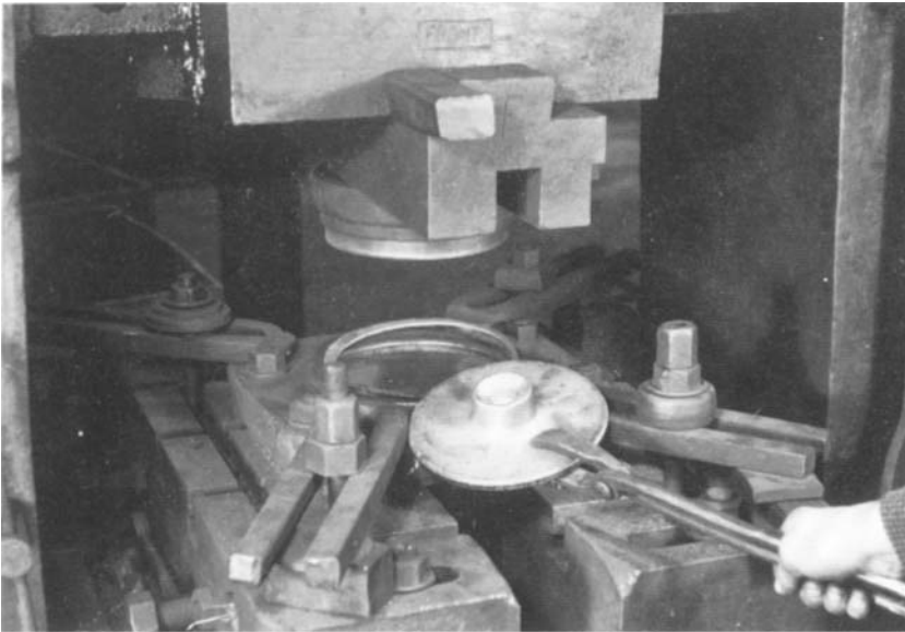
11.13 Flash trimming die deposited with Co-Cr-W alloy (courtesy Deloro Stellite Group).
