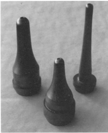
11.14 Glass plungers coated with Ni-Cr-Si-B alloy 40 RC by spray fusing (courtesy Deloro Stellite Group).
