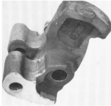
11.32 Manufacture of high speed train couplings incorporates coatings on the rubbing surfaces exposed to unlubricated wear and impact. The coating is a thermally sprayed layer of Ni–Cr–Si–B alloy containing tungsten carbide, which is then furnace fused. The lifetime is raised typically from three months to six years or more (courtesy British Rail).
