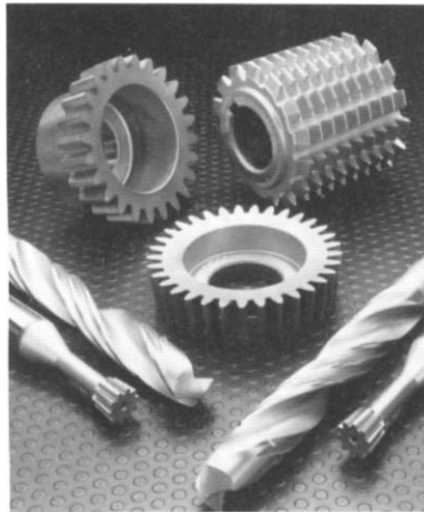
6.12 A selection of tools coated with TiN by ARE (courtesy Tecvac Ltd).
