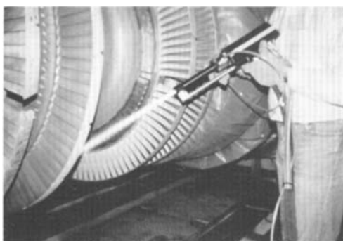
11.24 A stationary turbine being sprayed using a JP5000 torch to deposit chromium carbide/nickel chrome to a thickness of 0.25 mm, to reduce wear and erosion (courtesy Eutectic Co. Ltd).
