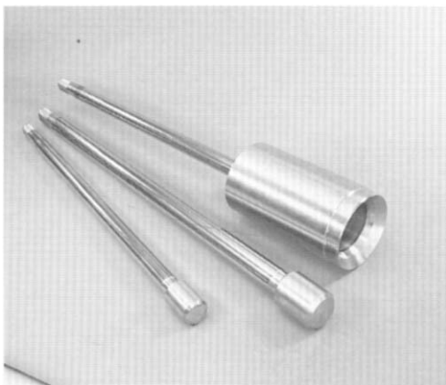
11.23 Steam turbine valve spindles coated by Jet Kote using chromium carbide and nickel chrome and with seat surfaces deposited with cobalt base alloys.
