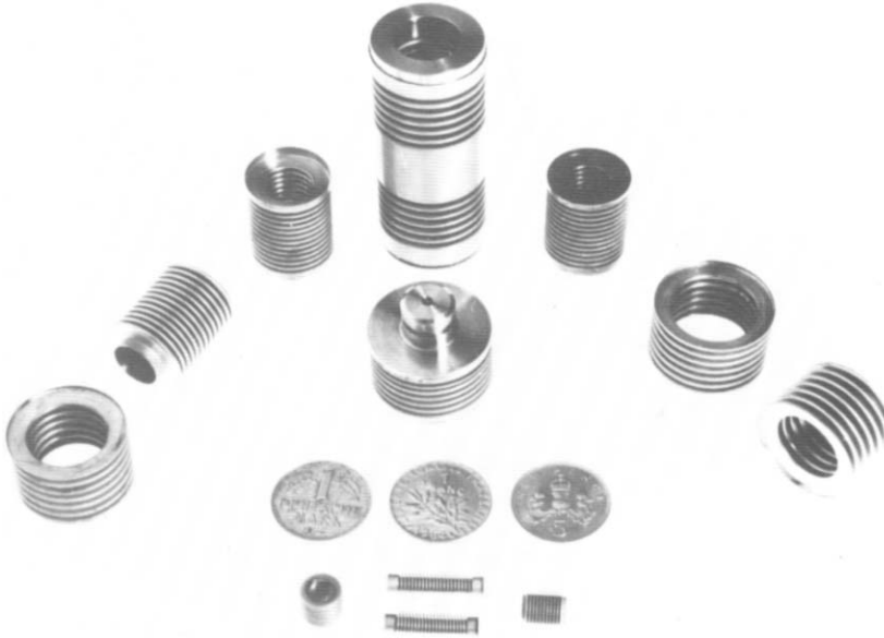
5.4 Miniature nickel bellows made by electroforming.
