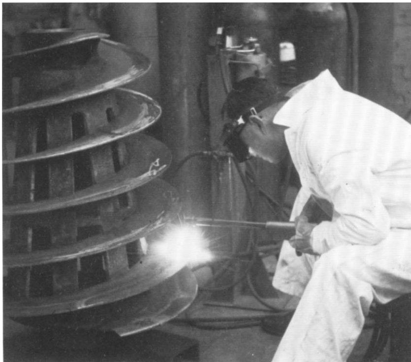
11.5 Centrifugal separator screw surfaced with cobalt alloys to resist abrasion and corrosion on the diameter and faces of the flights (courtesy Deloro Stellite Group).
