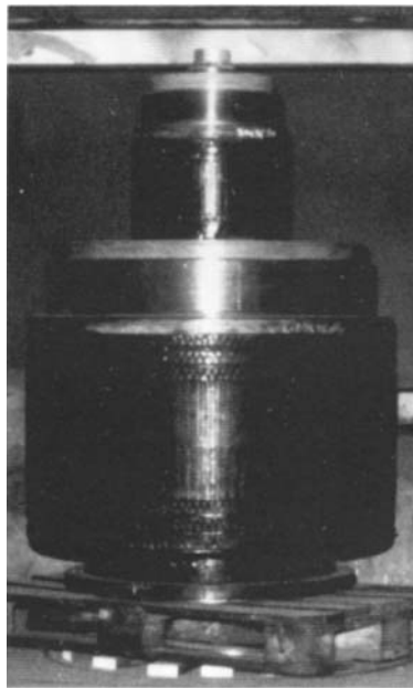
11.33 Rail traction motor shaft bearing seating reclaimed with a gas or arc sprayed deposit of martensitic chromium (13%) steel, before machining to size (courtesy British Rail).
