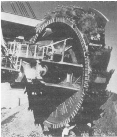
11.8 Extensive use of engineering coatings extends the life of the toothed buckets on this excavation unit (courtesy ESAB Group (UK) Ltd).
