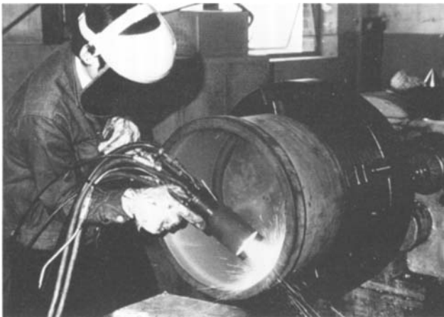
11.31 Reclamation of a passenger bus brake drum by arc spraying an initial coating of molybdenum, followed by a working layer of low alloy steel (courtesy Metallisation Ltd).
