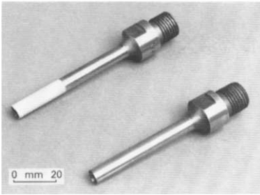
11.17 Paper drills plasma arc sprayed with tungsten carbide–cobalt material to a thickness of around 0.05 mm (courtesy CSIRO, Australia).
