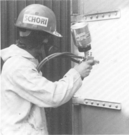
7.1 Magnum torch for plastics coating, designed for touch-up work on damaged components and for site work. The powder consumable is held in the torch-mounted hopper (courtesy Croboride Ltd).
