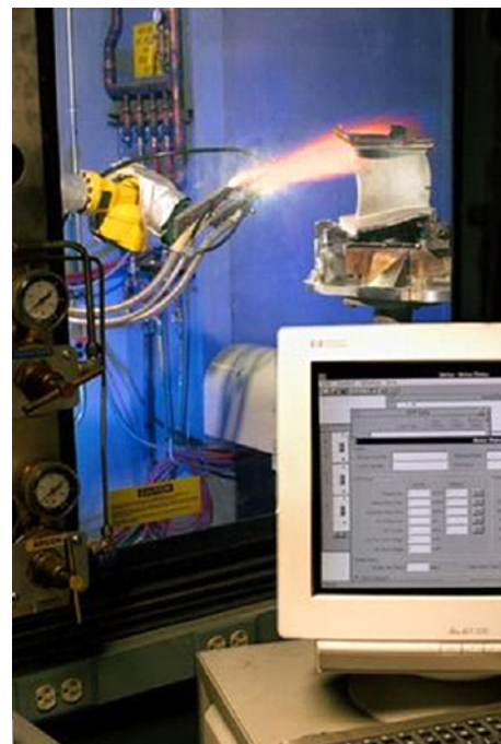
Fig. 2 An example of air plasma spraying (APS) in action, showing the gun end of the spraying robot, plasma plume, part being sprayed, and controls
